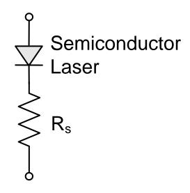
• The resistor R<sub>s</sub>, dampens current oscillations due to parasitic inductances in the circuitry
