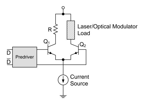
The predriver conditions the signals for input to transistors Q<sub>1</sub> and Q<sub>2</sub>
