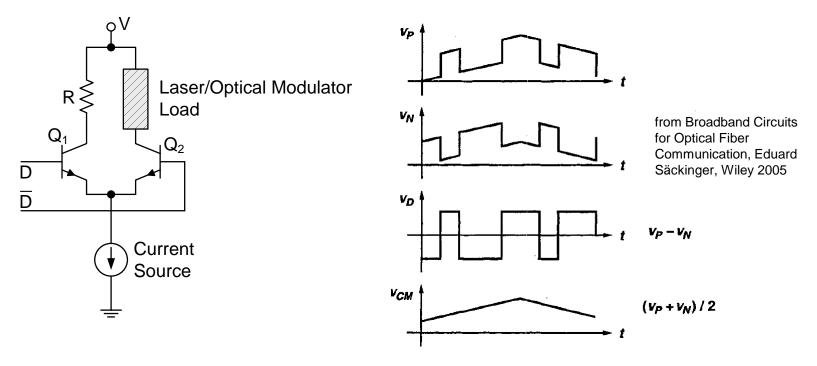
The differential design is insensitive to common-mode noise and avoids the need for an input reference voltage
