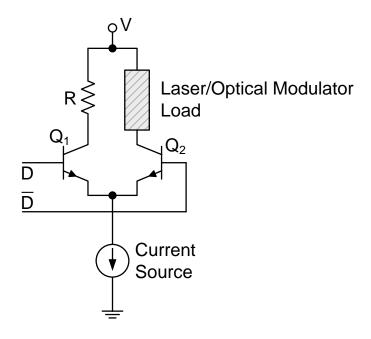
A constant current to the ground through the current source avoids current transients due to parasitic capacitances and inductances
