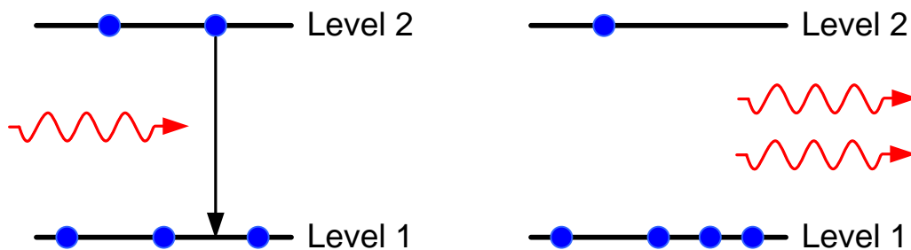
Figure 5. A Photon stimulates a particle to a lower energy level, creating a second photon.
