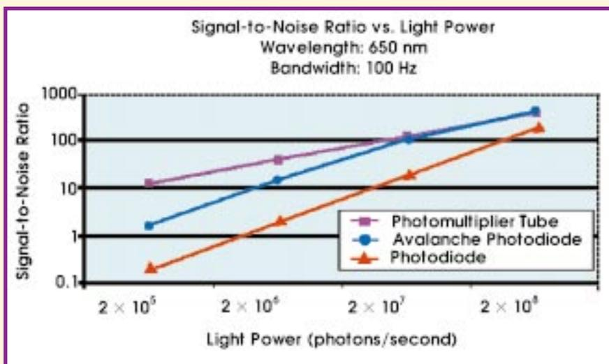
**Figure 4.** Avalanche photodiodes fill an application space between photodiodes and photomultiplier tubes in terms of signal-to-noise ratio and ability to operate at high or low light levels. As the wavelength or bandwidth changes, these curves will change.
