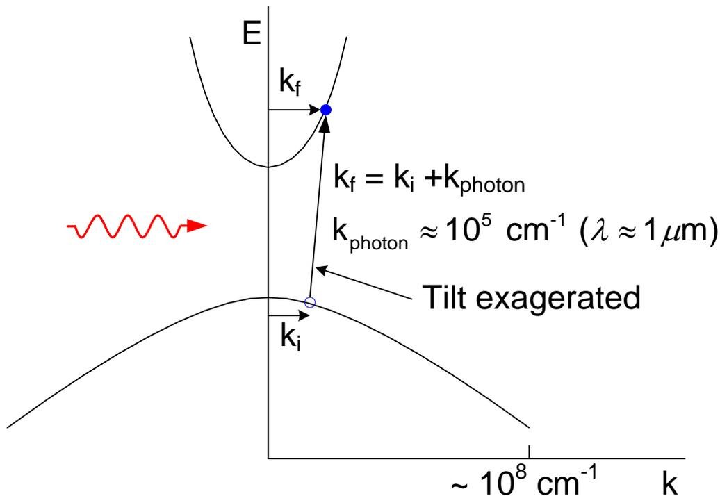
Figure 11. Optical transitions in semiconductors are “vertical”.
