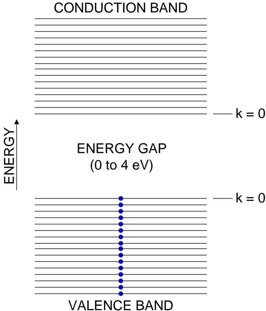
Figure 8. Energy bands in a semiconductor
