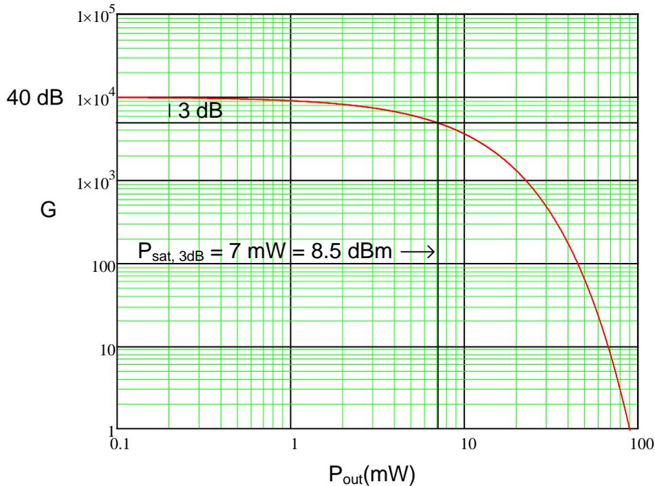
Figure 10. Gain as a function of amplifier output.
