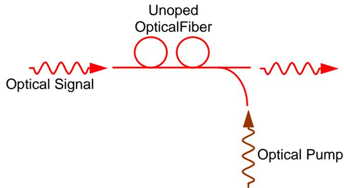
Figure 4. A fiber Raman optical amplifier.
