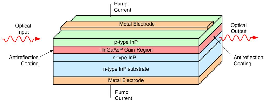
Figure 3. A semiconductor optical amplifier.
