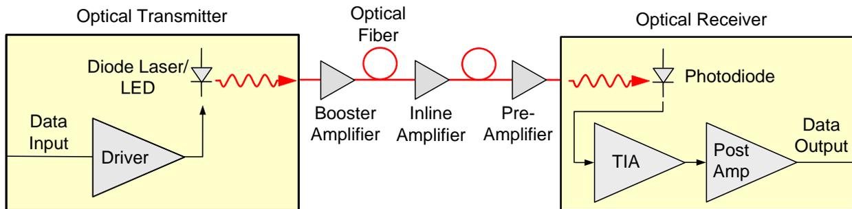
Figure 1. Optical amplifiers in a fiber optic data link.
