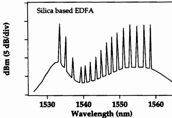
Figure 11. Simultaneous amplification of 16 optical signals by a chain of 4 EDFAs. [From *Erbium-Doped Fiber Amplifiers: Fundamentals and Technology*, P. C. Becker, N. A. Olsson, and J. R. Simpson, (Academic Press San Diego, 1999), p. 290; after B. Clesca et al. *Electron. Lett.* Vol. 30, pp. 586-587]
