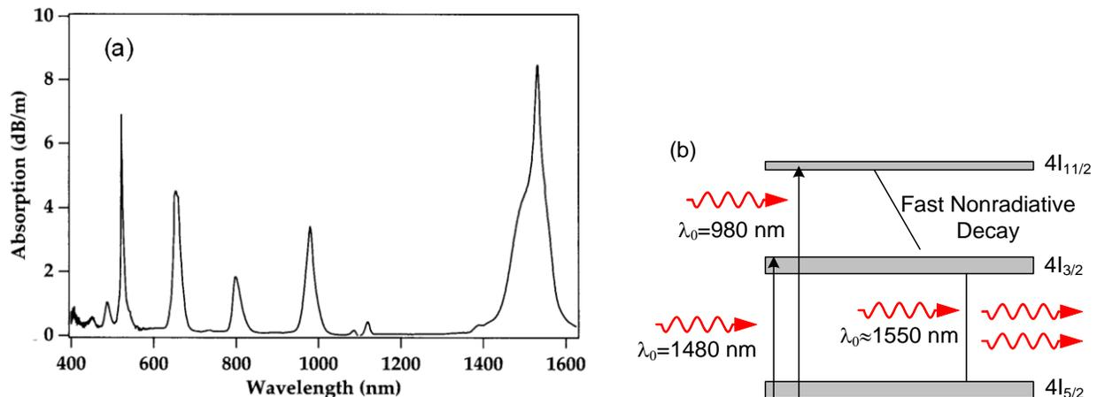
Figure 8. (a) Absorption for an erbium-doped glass fiber. The absorption in the region from 400 to 600 nm has been divided by 10. [from *Erbium-Doped Fiber Amplifiers: Fundamentals and Technology*, P. C. Becker, N. A. Olsson, and J. R. Simpson, (Academic Press San Diego, 1999), p. 112] (b) Optical transitions between energy levels that result in the absorption pictured in (a).
