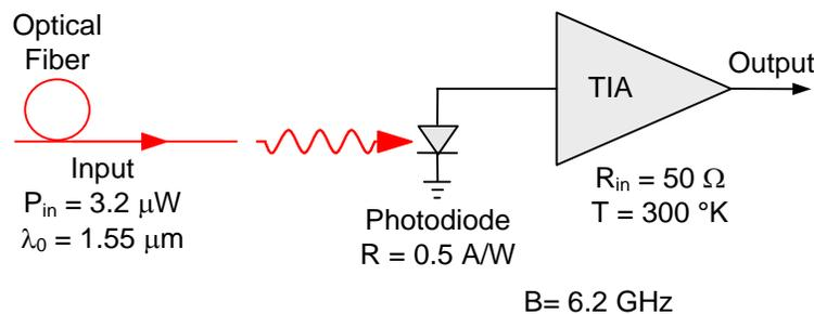
Figure 12. An optical receiver without an EDFA optical pre-amplifier.
