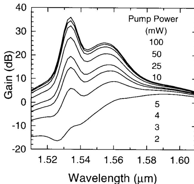
Figure 7. Gain for an erbium-doped fiber amplifier. The pump wavelength is 1480 nm, the fiber length is 30 meters, and the input signal power is -30 dBm. [From *Optical Amplifiers*, Mikhael N. Zervas and Gerlas van den Hoven, Chapter 5 in *Fiber Optics Communication Devices*, Norbert Grote and Herbert Venhhaus, Editors, (Springer, Berlin, 2001) p. 169]
