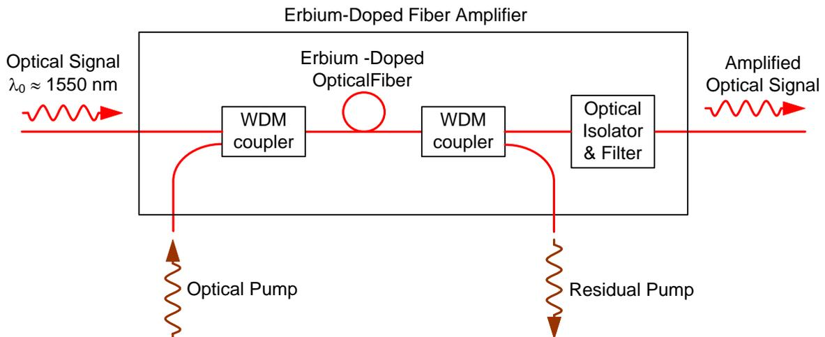
Figure 5. An EDFA for which the optical signal and optical pump are co-propagating.
