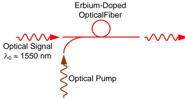
Figure 2. An erbium-doped fiber amplifier.
