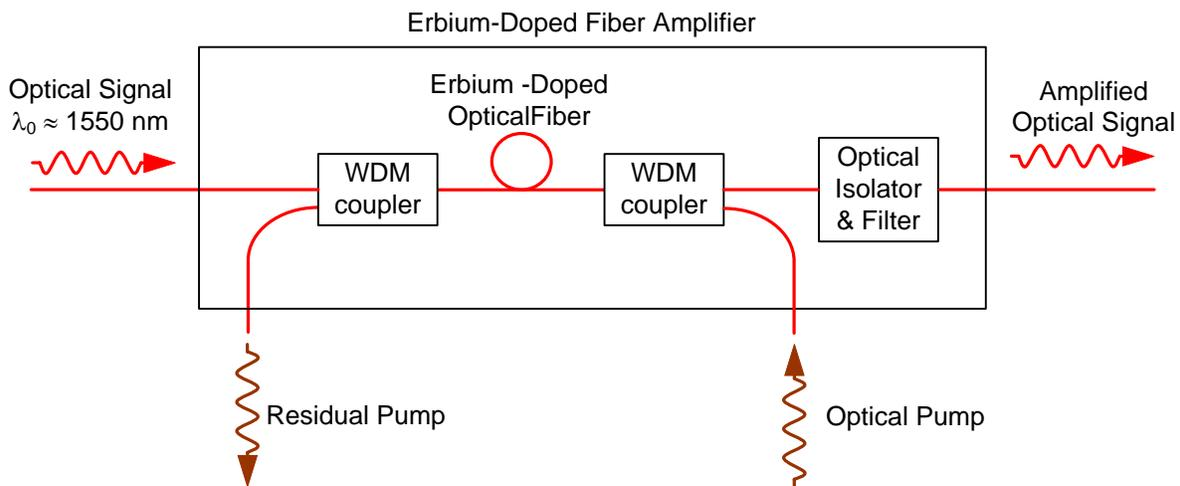
Figure 6. An EDFA for which the optical signal and optical pump are counter-propagating.
