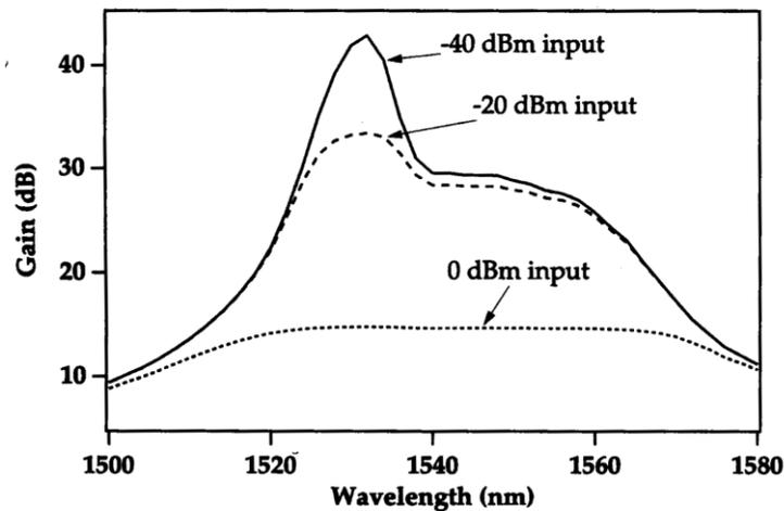
Figure 9. Simulated gain versus signal input level for an EDFA with 10 meters of optical fiber, pumped with 50 mW at 980 nm. [from *Erbium-Doped Fiber Amplifiers: Fundamentals and Technology*, P. C. Becker, N. A. Olsson, and J. R. Simpson, (Academic Press San Diego, 1999), p. 282]
