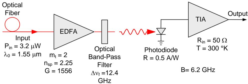
Figure 13. An optical receiver with an erbium-doped fiber pre-amplifier.
